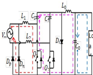
Figure 3(a). Mode 0 operation during positive half-cycles of the supply voltage
