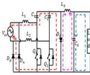
Figure 3(b). Mode 1 operation during positive half-cycles of the supply voltage
