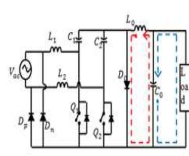
Figure 3(c). Mode 2 operation during a complete switching period for the positive half-cycles of the supply voltage
