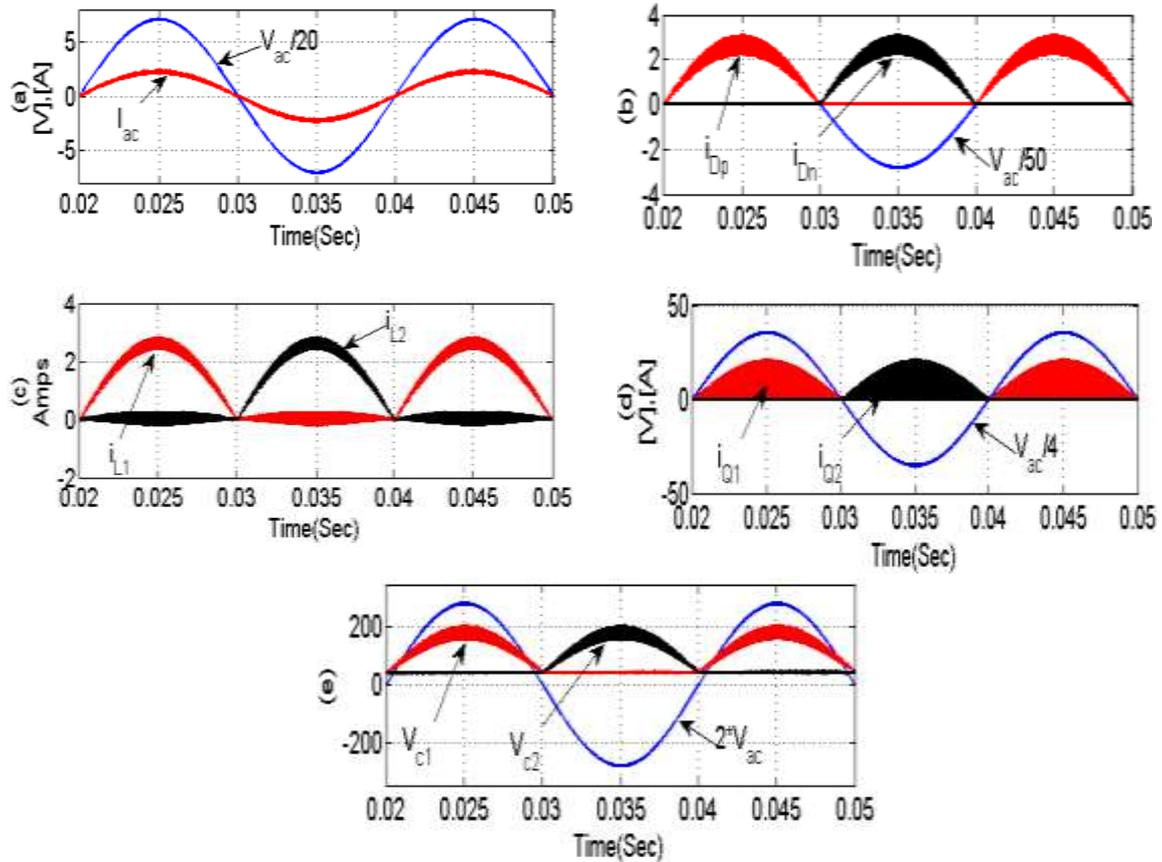
Figure 7(a -e). A sinusoidal supply current in phase with supply voltage
