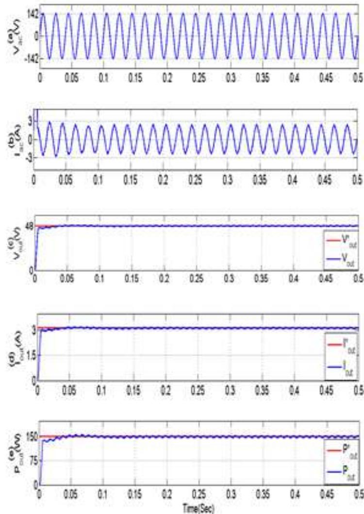
Figure 6(a)-(e). The proposed converter operating at rated supply voltage of (141.4 V)
